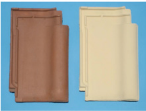
Figure 9: Crude red-brick ( \beta_s = 0.53 ) and painted one (bright brown, \beta_s = 0.30 ) [13]
